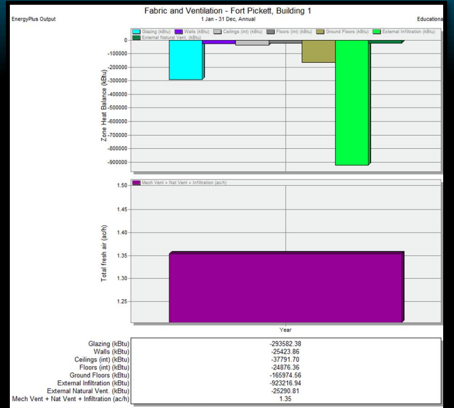
HEAT TRANSFER FOR ENCLOSURE
